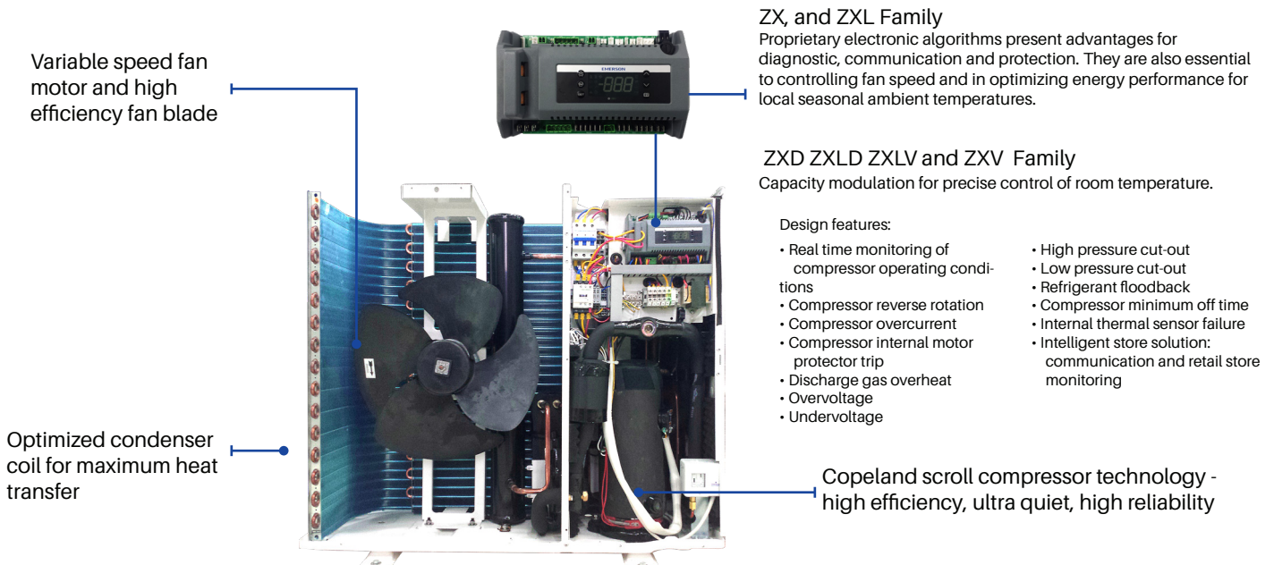
Figure 1. Copeland ZX Platform CDU features
